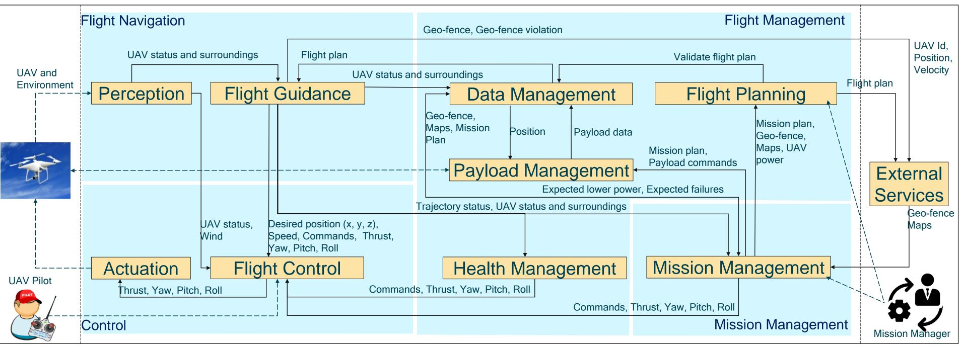
\*UAV status: Actual Position, Attitude, Velocity, Power Level, Engine(s) status, ...
