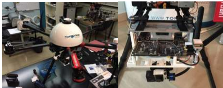
Figure 54 - UC5 D1: TopView MANTIDE 900 with no payload and with a high-performance onboard computer prototype payload based on Nvidia Jetson
