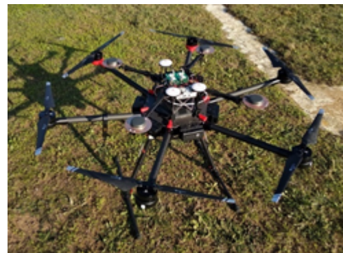
b. Integration of GLAD+ on drone platform.
