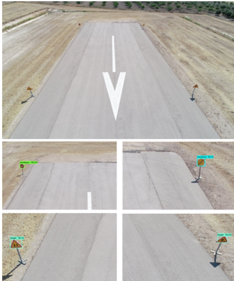
Figure 43: Detections performed by Faster R-CNN on a Drone Flight image. (top) The model fails to perform any detection over the whole image. (bottom) After chopping the image, the model correctly detects and identifies the four traffic signs.
