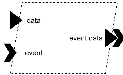
Figure 5: Ports in a thread, with "data" and "event" as inputs and "event data" as an output
