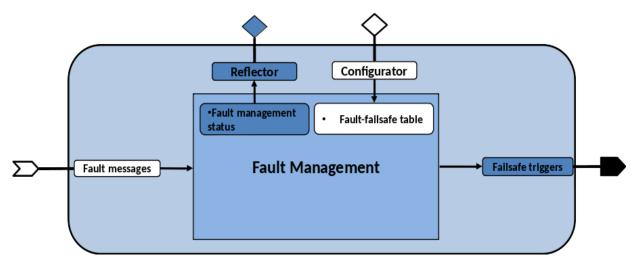
Figure 47: Fault Management block model
