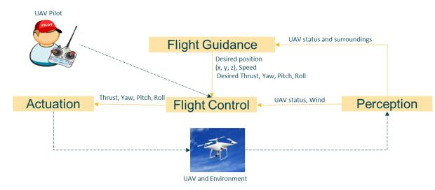
Figure 13: Guidance, navigation, and control pattern
