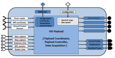
Figure 30: HSI payload management block
