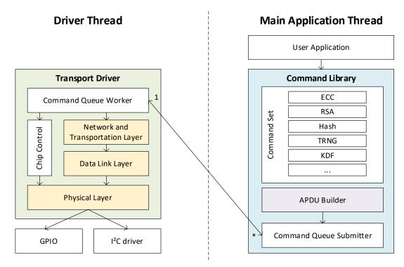
Figure 33: Design of generic architecture and SW-API for integrating various HSM modules into a drone
