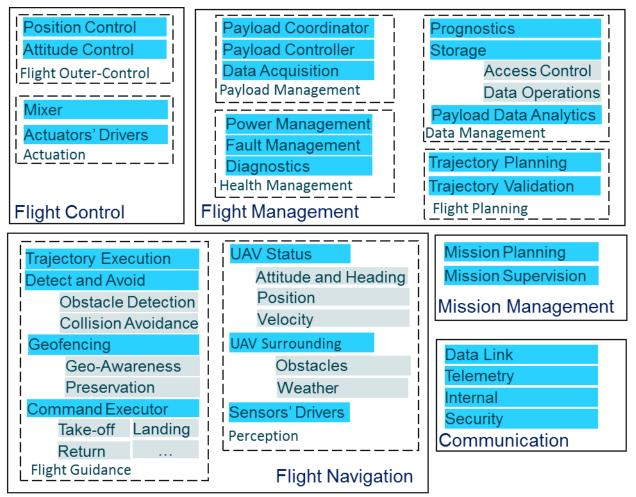
Figure 26: Clusters of the reference architecture building blocks
