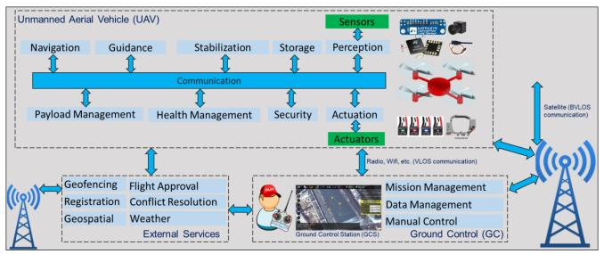
Figure 5: The building blocks of UAS and their interactions with external services
