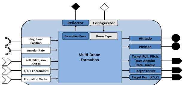
Figure 35: Multi-drone formation block model
