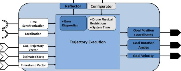
Figure 37: Trajectory execution block model
