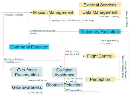
Figure 11: Detect and avoid and geofencing patterns
