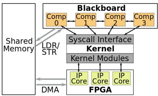
Figure 28: Blackboard pattern for managing the complexity of SoCs
