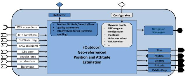
Figure 32: Outdoor positioning system block
