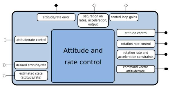
Figure 42: Attitude and control block model
