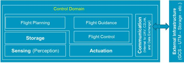
State Modelling: Storage (geo-fence, plans, etc.) and Perception (flight data acquisition and analysis)
