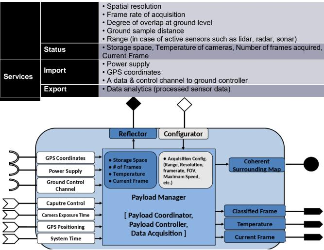
Figure 49: Payload coordinator block model
