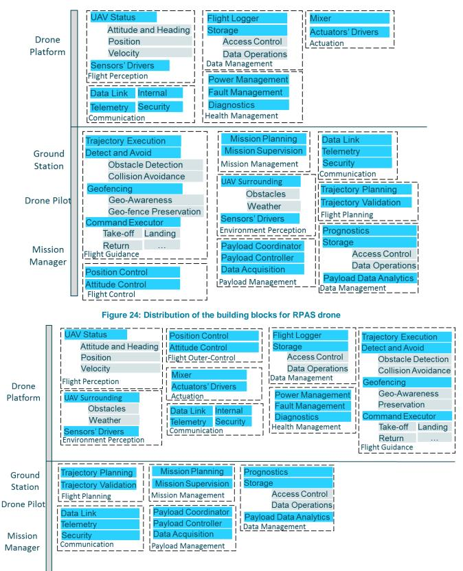
Figure 25: Distribution of the building blocks for semi-autonomous drone
