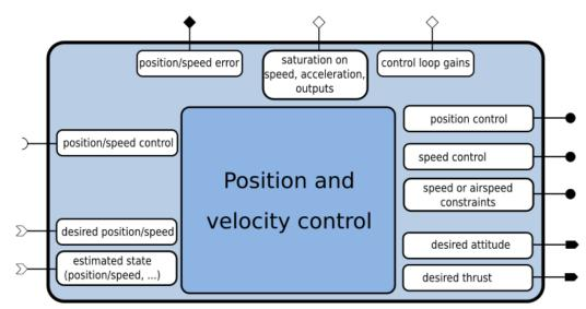
Figure 41: Position and velocity control block model
