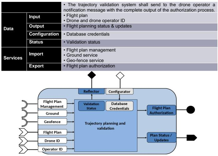
Figure 36: Trajectory planning and validation block model
