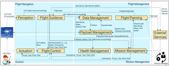
\*UAV status: Actual Position, Attitude, Velocity, Power Level, Engine(s) status, ... \*UAV surrounding: Wind, Temperature, Static and dynamic obstacles, ...
