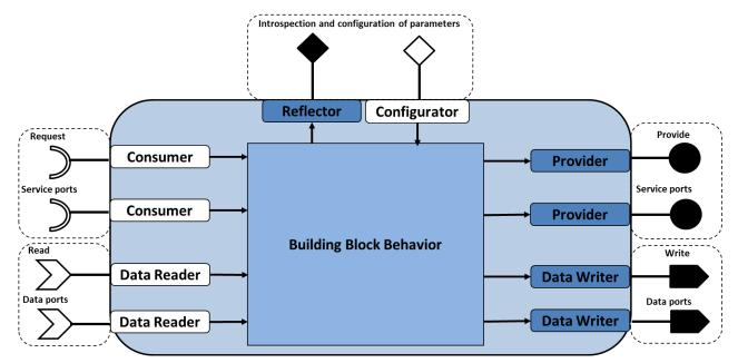
Figure 4: A template for the architecture generic blocks
