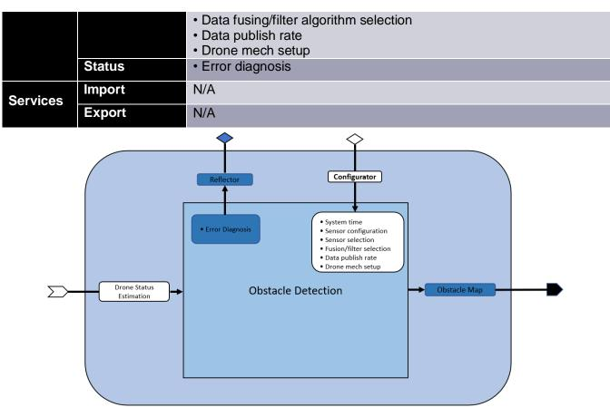
Figure 38: Obstacle detection block model
