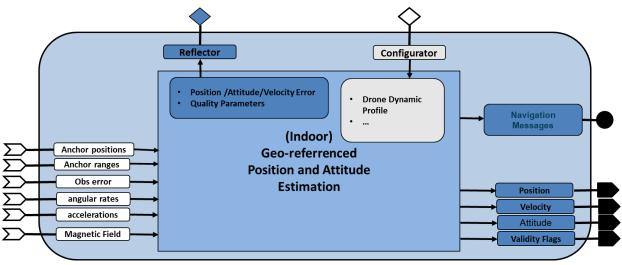
Figure 31: UWB-based indoor positioning system block
