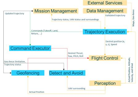
Figure 10: Flight guidance pattern
