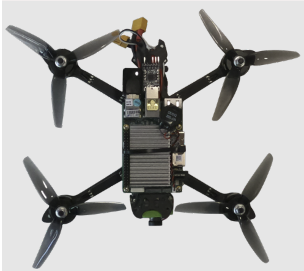
Figure 24 Top view of the proposed MAV UC4-D2-FUN-05 – Vehicle platform equipped with all sensors (event-based camera, micro lidar) and electronics (Intel Up Core), as exploited for output generation in TUD contribution to COMP12 WP4-01. Credits: Julien Dupeyroux (MAVLab, Delft University of Technology).
