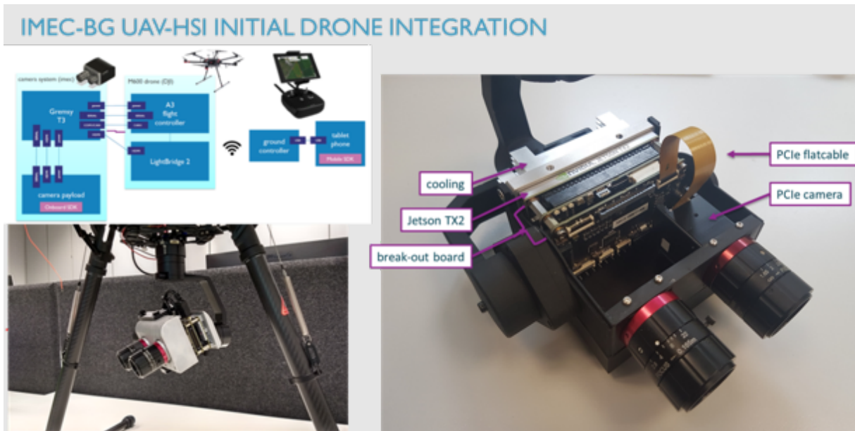
Figure 21: Example prototype payload and a possible integration with a DJI M600 drone
