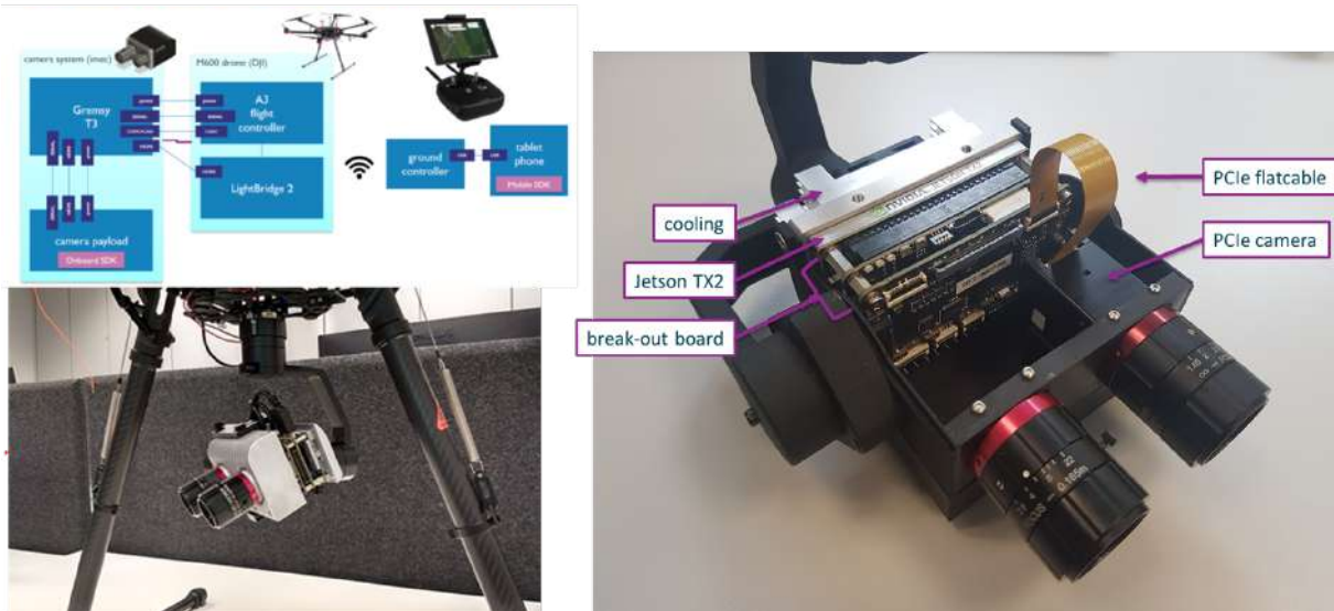
Figure 23: Example prototype payload and a possible integration with a DJI M600 drone
