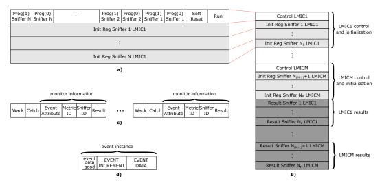
Fig. 6. Data organization in the proposed monitoring system: a) control and initialization registers of the LMICs; b) DCI register space; c) structure of the sniffer output; d) structure of an event instance.
