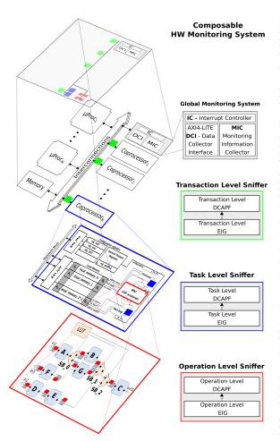
Fig. 9. Example of the proposed HW Monitoring System.
