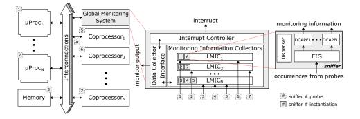
Fig. 5. HW block diagram of the complete monitoring system applied to the considered reference architecture.
