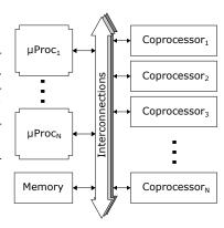
nection buses. Here with coprocessors we intend dedicated Fig. 1. Baseline reference architecture. hardware accelerators, which can be either fixed function or reconfigurable ones, loosely coupled
