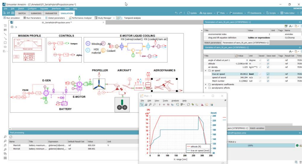
Figure 1: Screenshot of Simcenter Amesim GUI. Flight performance Simulation of a serial hybrid propulsion aircraft.
