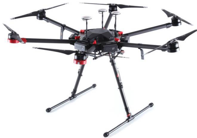
Figure 48: Off-the-shelf multi-rotor platform with 5Kg payload
